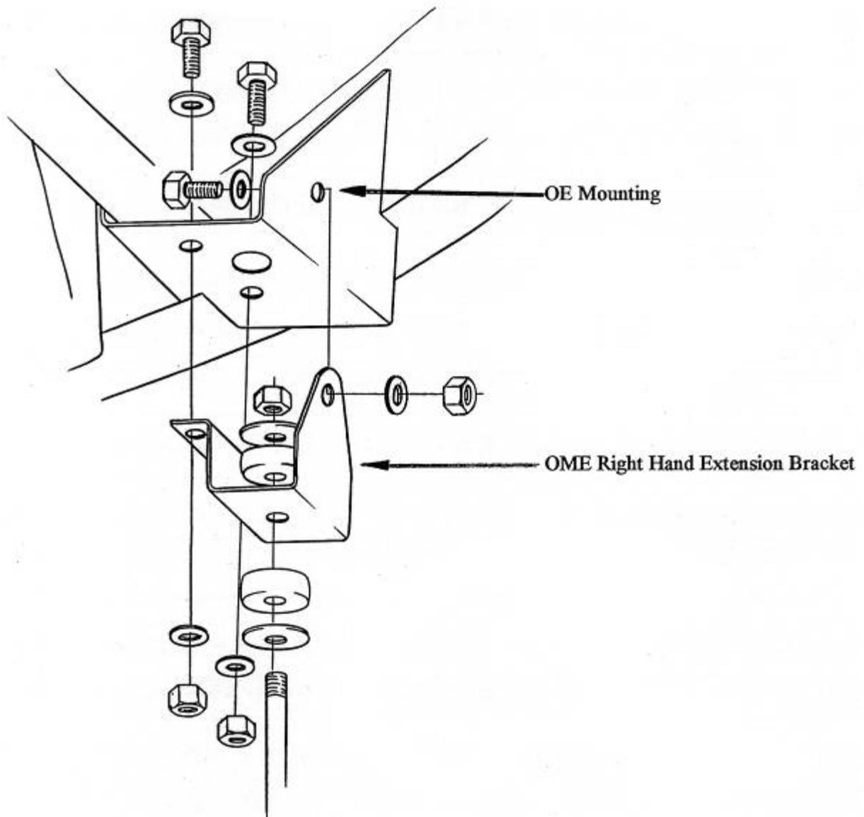
3. Place right hand OME extension bracket up against OE mount (as per Diagram No. 2) aligning the two holes that mount the sway bar extension arm and clamp in position. Using an 8mm bit, drill the three original mounting holes and securely bolt together using the 8mm bolts, nuts and washers supplied.
