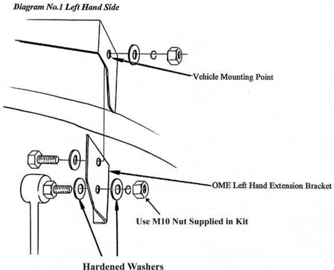
2. Place OME left hand extension bracket inside the vehicle mounting point using the 10mm bolt supplied and tighten securely.
